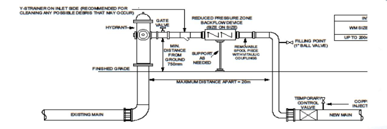
Schematic of temporary connection from watermain with Backflow Prevention using a CSA-certified reduced pressure principle backflow
